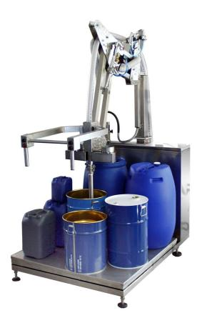
Drumming with semiautomatic machine operator. The machine can perform 120/200L filling drums on pallets, drums 25/30/60 liter narrow mouth wide or individually or on pallets, the particular shape of the mobile arm centering makes the operation manual in the mouth of the container particularly agile and fast.
